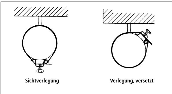
Conductor Holder Type PV
