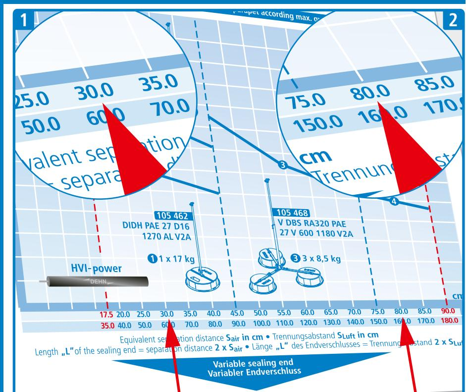
Determining the equivalent separation distance **Sair** using the table
