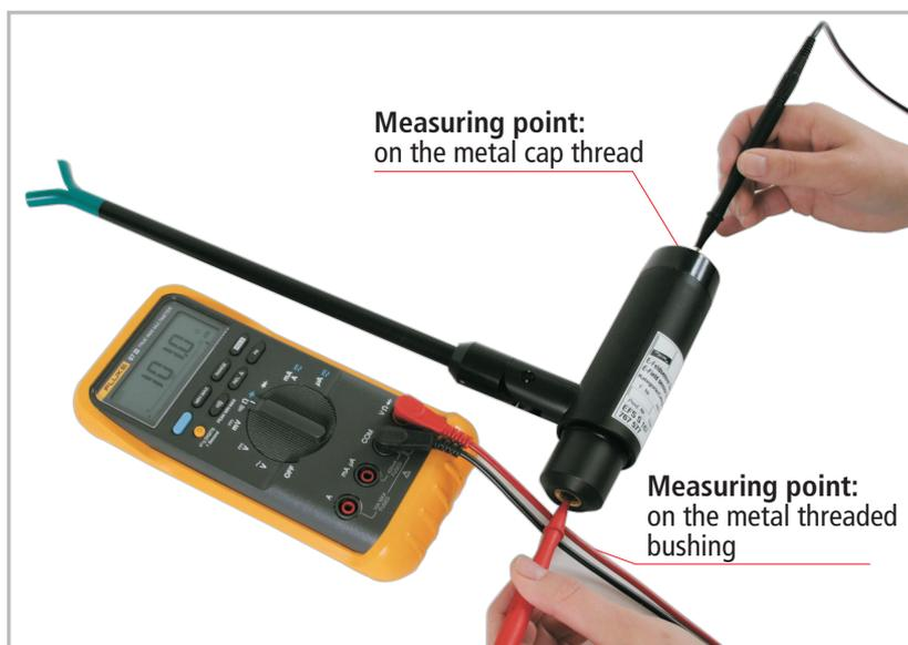
Fig. 3.2.11 Testing an electric field sensor for correct operation
