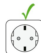
socket outlet with earthing contact
