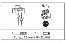
The remote status indicator (SPDT contact) shall be connected to NEC class 2 circuits only!
