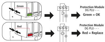
Testing Remote Contact Signaling (with modules installed)
