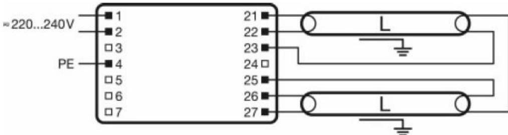
Max. permitted cable length between ECG and lamp: 1.5 m
