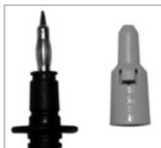
Only with mounted safety cap on the test electrode of the measuring line tests in CAT III environments are permitted in accordance with EN 61010-031.
