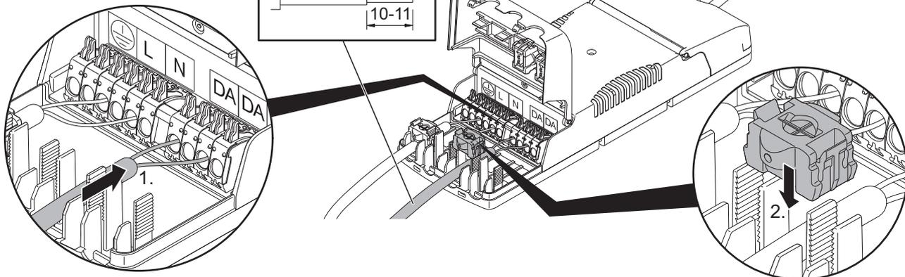
15 **Looping-in (feed through) - Durchschleifen**
