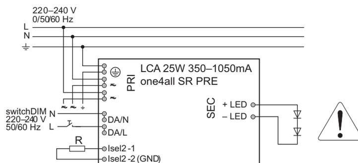
12 **EN** Connect the power cable to the driver.
