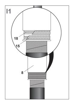
Abrade, degrease and clean the cable outer jacket (110), the cable gland (8).
