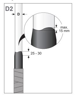
**Chamfer the outer semicon layer** in between 25 to 30 mm.
