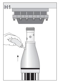
Remove the temporary protection from the connector stud. Clean and degrease the transparent cover part of the silicone stress cone (12) with alcohol.
