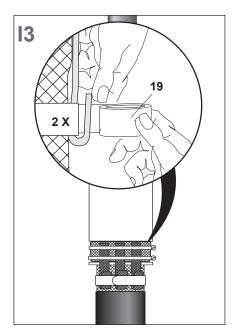
Connect the lower ends of the copper braids (24) to the lead sheath with a roll spring (19). Apply two turns of the roll spring, bend back the copper braids, then apply the rest of the roll spring.
