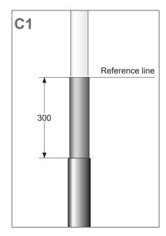
Remove the outer jacket (110) and bedding 300 mm below the reference line.
