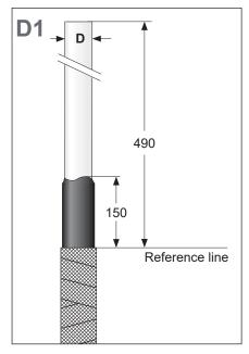
Thoroughly remove the outer semicon layer (104) to within 150 mm above the reference line until the diameter of the insulation (103) is D (see Table 1).
