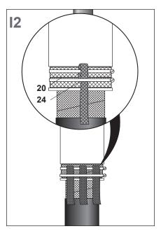
Remove the PVC tape. Fix the three copper braids (24) to the shield wires as shown using two armour clamps (20).
