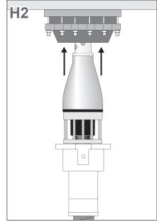
Push the cable with the male plug-in unit in a straight line into the epoxy insulator (5).
