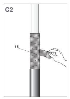
Apply three layers of copper mesh tape (15) onto the lead sheath (107).
