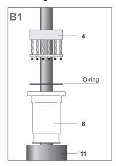
Move the heat shrinkable thick wall tubing (11), cable gland (8), O-ring and compression device (4) down the cable jacket as shown in the drawing.
