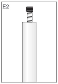
Protect the conductor (101) with PVC tape (23) as shown.
