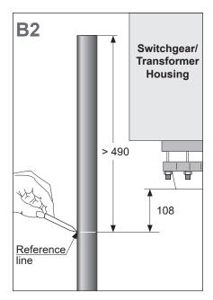
Mark the reference line on the cable 108 mm below the transformer switchgear housing as shown.
