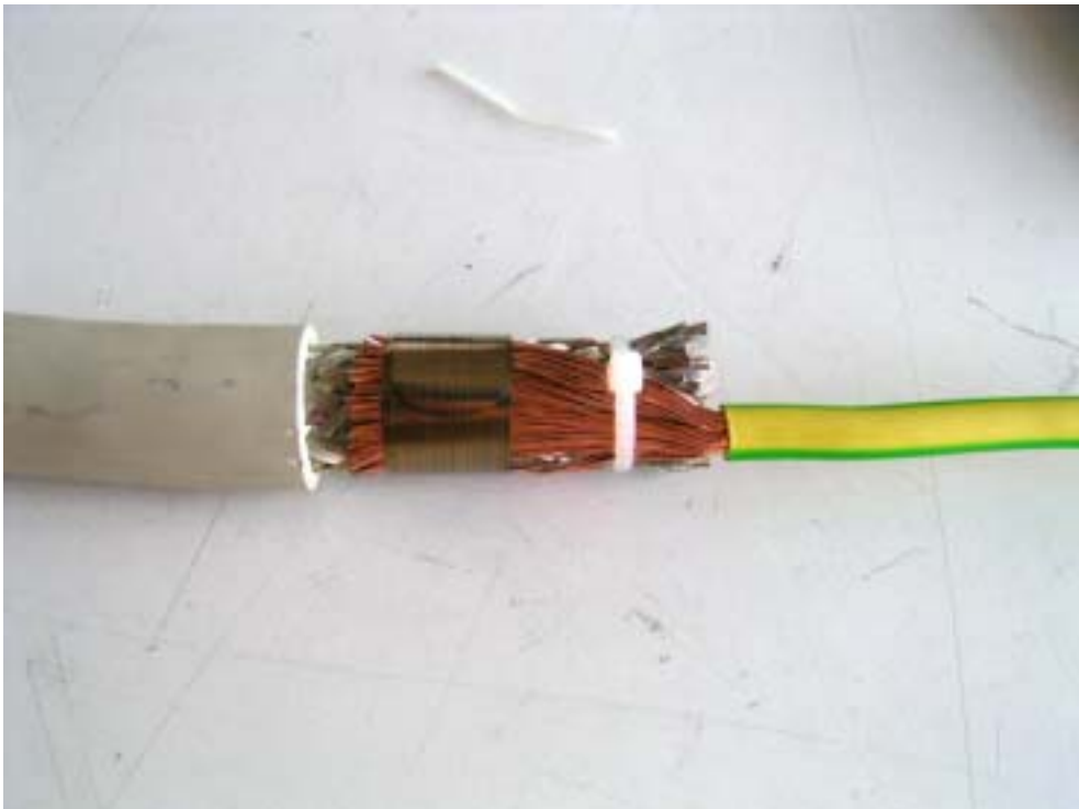
Fig. 3.4: Contact force spring complete mounted; for better stabilisation this could be fixed with a cable tie
