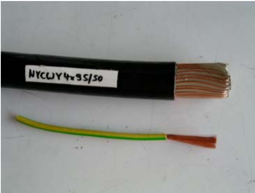
Fig. 1.1: Remove the insulation of e.g. NYCWY 4x95/50 cable (for contact force spring SA KRF 50 V2A and PE 1x16 mm 2 conductor (stranded) by approx. 5 cm in length.
