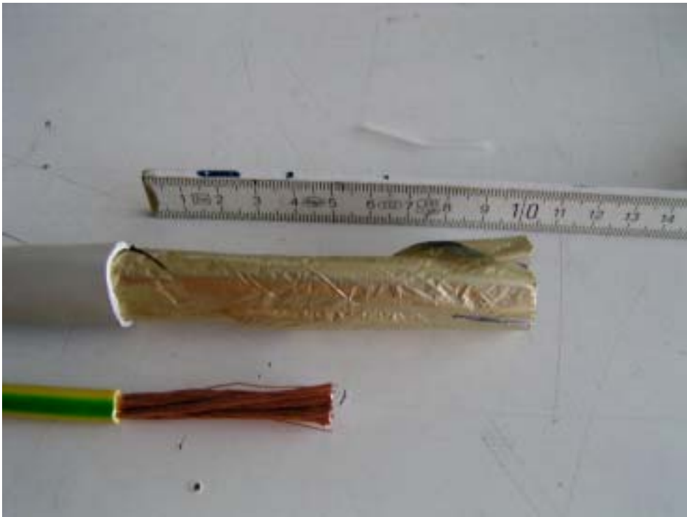
Fig. 4.1: Remove the insulation of e.g. JE-Y(ST)Y 40x2x0.8 cable for contact force spring SA KRF 22 V2A by approx. 10 cm and PE conductor 1x16 mm \leq (stranded) by approx. 5 cm in length.
