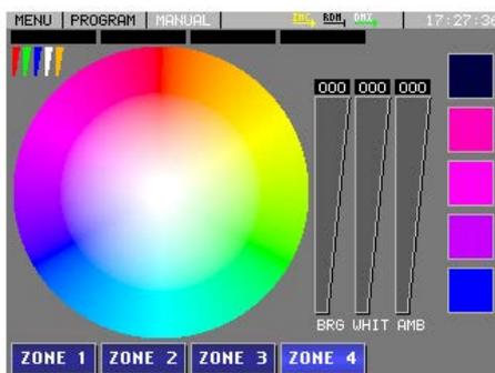
RGBAW: The RGBWA mode has 5 channels. In slider mode you can set the channel value with the sliders separately. In Palette mode you can select color from the palette. Each color on the palette consist of all the 3 primary colors (RED, GREEN, BLUE) and two additional color (WHITE and AMBER), and one of them is always 100%.
