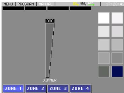
**DIMMER:** The DIMMER has only one channel. Its value can be set with one slider.
