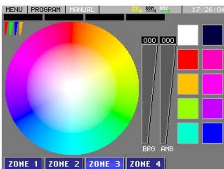
**RGBA or RGBW:** The RGBA or RGBW mode has 4 channels. In slider mode you can set the channel value with the sliders separately. In palette mode you can select a color directly from the palette. Each color on the palette consist of all the 3 primary colors (RED, GREEN, BLUE) and an additional color (AMBER or WHITE), and one of them is always 100%.
