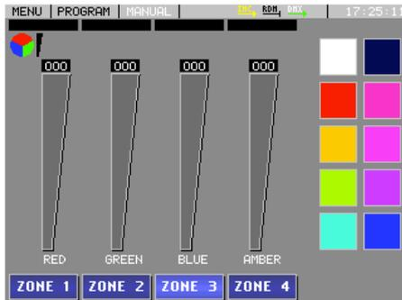
To regulate the selected color to 0% you can do it by BRIGHTNESS slider. There is also a third mode to select a color, it is a mixed palette and slider selection. The RGB can be select by palette and the amber or white color has its own slider.
