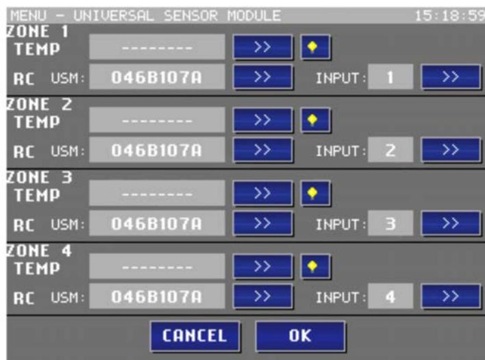
Two different features can be programmed in this menu: a temperature sensor and a remote controller.
