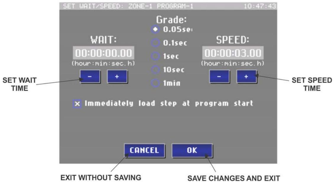
Touch the **SET WAIT/SPEED BUTTON** to open the set wait/speed window. On the left side the WAIT time can be adjusted with the '+' and '-' buttons. On the right side the SPEED time can be adjusted with the '+' and '-' buttons. In the center of the screen the changing range can be selected. The maximum selectable time can be 2 hours.
