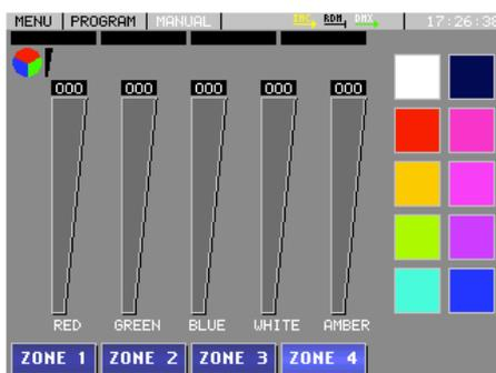
To regulate the selected color to 0% you can do it by BRIGHTNESS slider. As in RGBA or RGBW Mode, there is a third mode to select color, it is a mixed palette and slider selection. The RGB can be select by palette and the white and amber color have their own sliders.
