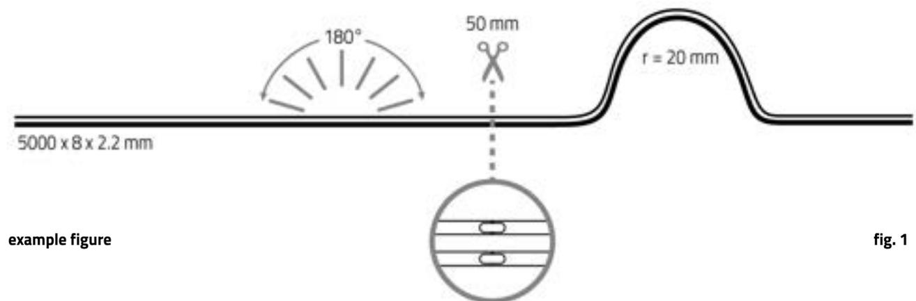
Separate the **VARDIFLEX** LED strip at the marked position. For a tightly assembled LED strip is a micro side cutter or an optional cutter required.
