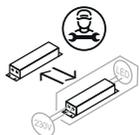
LED control gear can be replaced by a qualified electrician.
