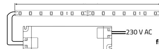
In the case of one-sided supply with a power supply unit, the LED strip can only be operated for a maximum of 5 metres at a time (fig. 2).
