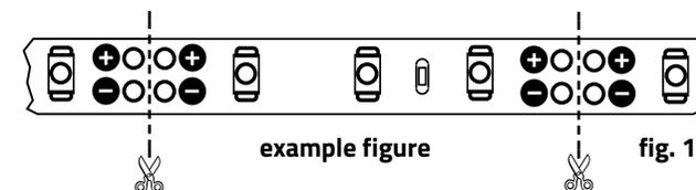
Separate the VARDAFLEX LED strip at the marked point. A micro side cutter or optional cutter is required for LED strips with a narrow!
