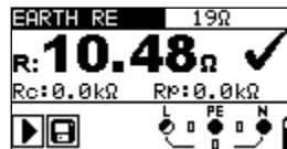
Figure 5.35: Example of an earthing resistance measurement
