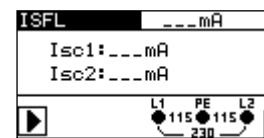
Figure 5.41: Single-fault leakage current (ISFL)
