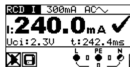
Figure 5.20: Example of a tripping current measurement
