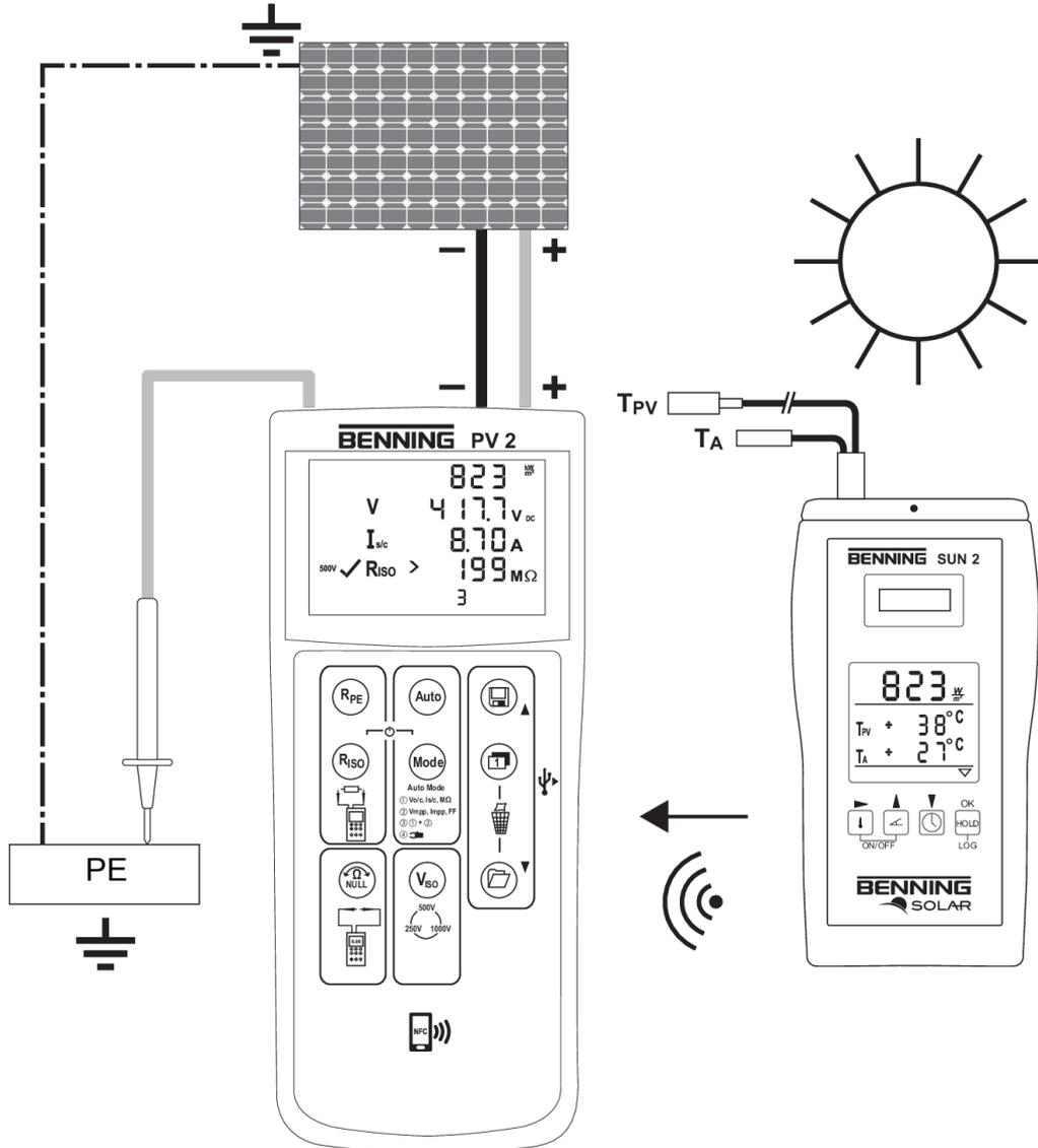
Figure 12: Radio connection to the BENNING SUN 2
