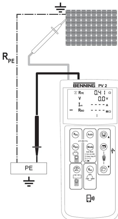
Figure 6: Protective conductor resistance measurement
