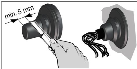
7. Insert cable grommet into housing.
