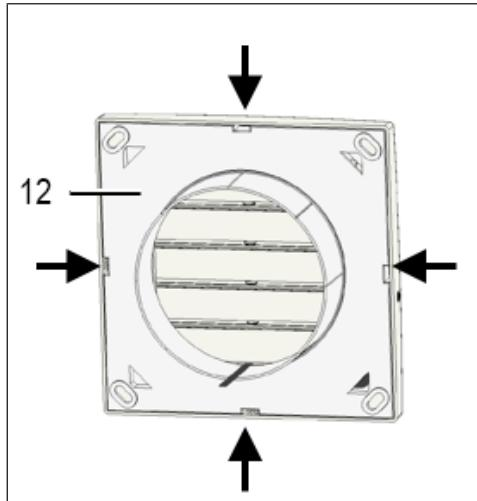
1. Unpack the external shutter with external combination sensor and remove the outer piece. To release the outer piece's locking hook, unlock (→ arrow) using a screwdriver.
