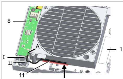
10. Insert housing into wall breakthrough/wall sleeve and secure with two screws. Do not insert the housing such that it is twisted or crushed. Make sure you use mounting material which is sized for the purpose.
