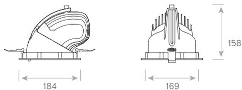
Abmessungen in mm / Dimensions in mm
