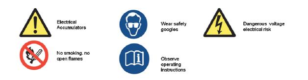
Labelling may vary due to application and dimension of the Battery. The manufacturer, respectively the importer of the batteries shall be responsible for placing the symbols (a minimum size is specified). In addition, consumer/user information on the significance of the symbols may be attached.
