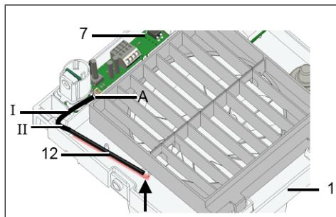
8. Insert housing into wall breakthrough/wall sleeve and secure with two screws. Do not insert the housing such that it is twisted or crushed. Make sure you use mounting material which is sized for the purpose.
