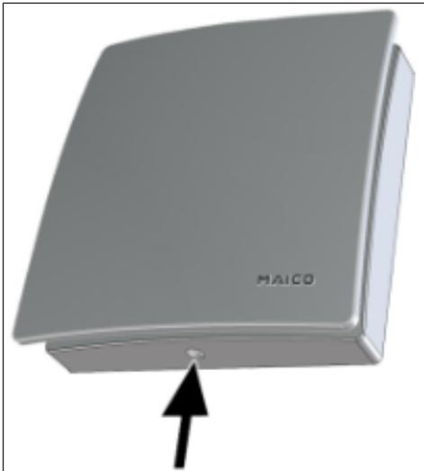
2. To release the cover's locking hook, unlock using a screwdriver.
