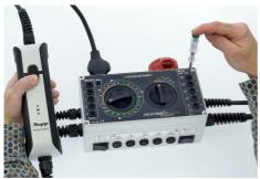
Repeat testing of the sensor surface with the PRCD-S pro mains plug rotated 180°.
