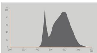
EPREL Data Spectral Diagram LEDr
