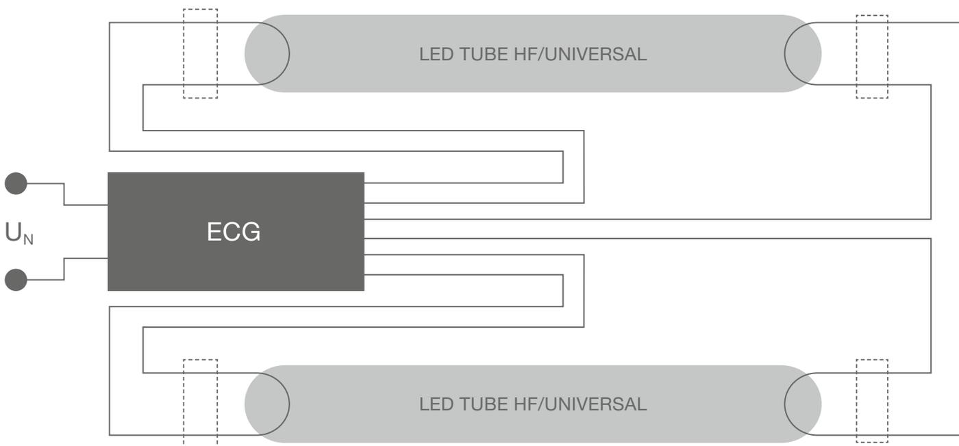
The wiring of the luminaire remains unchanged after retrofitting with LED TUBE HF/UNIVERSAL.
