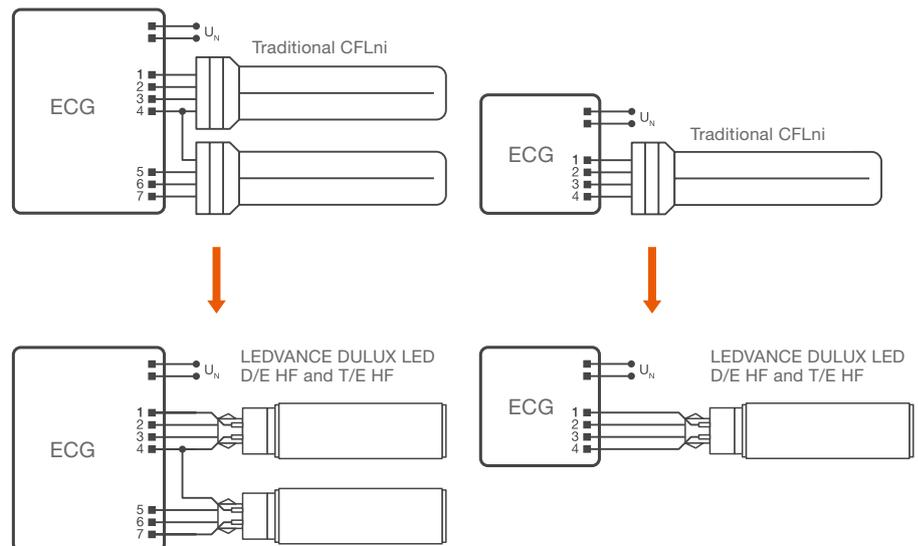
LEDVANCE DULUX LED D/E and T/E HF are not suitable for operating on electromagnetic control gear (CCG).
