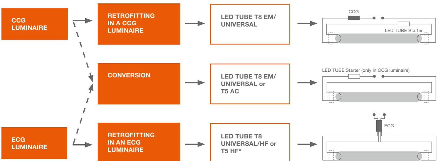
\* Check ECG compatibility at [ledvance.com/ecg-compatibility](http://ledvance.com/ecg-compatibility) or [ledvance.com/tubefinder](http://ledvance.com/tubefinder)
