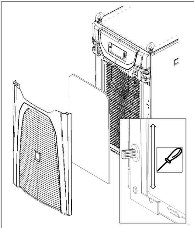
Fig. 35: Insert the textile filter mat 3319100, 3320200 and 3334300
