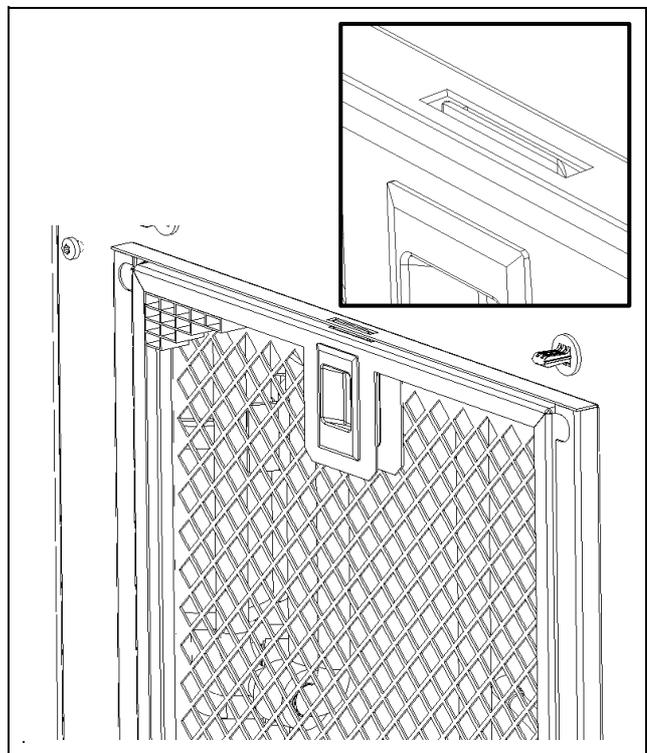
Fig. 37: Press in the metal filter 3319100, 3320200 and 3334300
