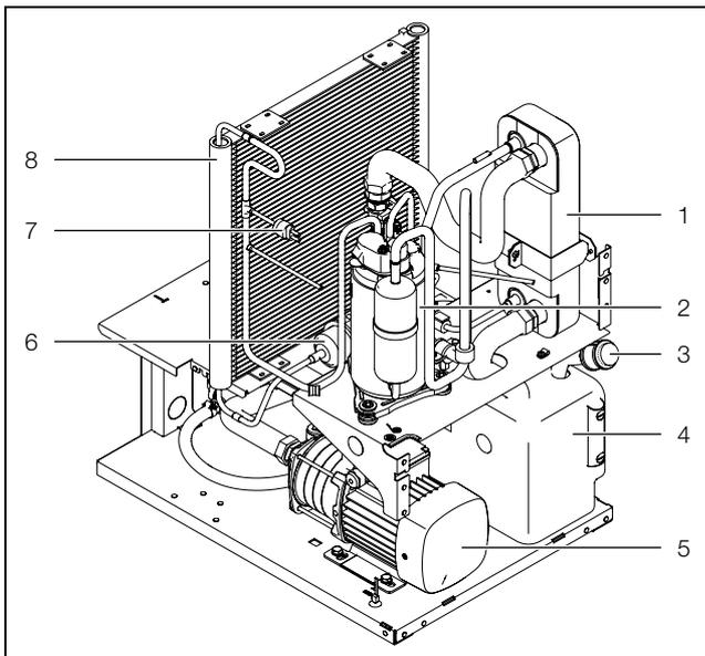
Fig. 7: Components inside the chiller
