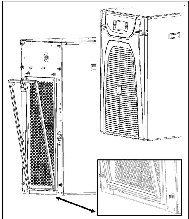
Fig. 36: Insert the metal filter 3319100, 3320200 and 3334300
