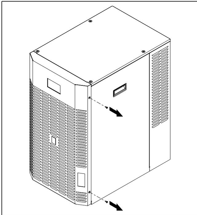
Fig. 14: Remove the locking screws
