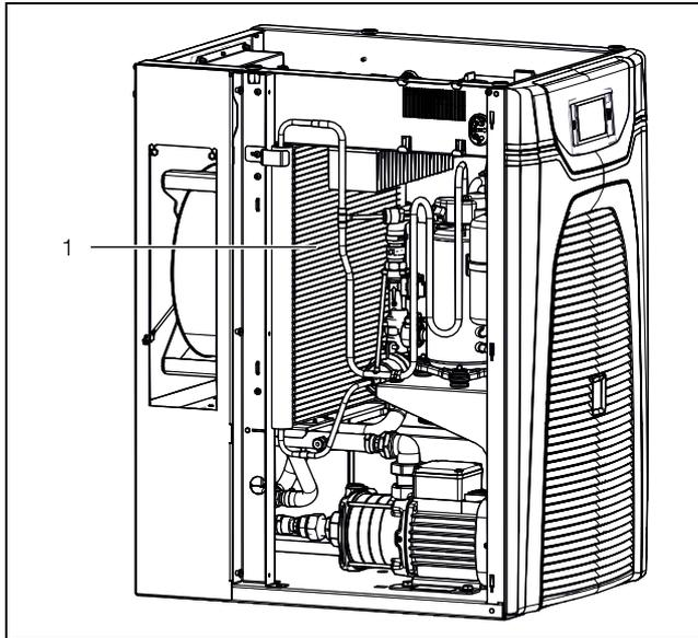
Fig. 51: Cleaning the condenser (shown here: 3334300)
