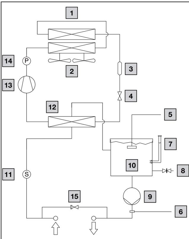
Fig. 10: Schematic diagram of refrigerant circuit 3334450
