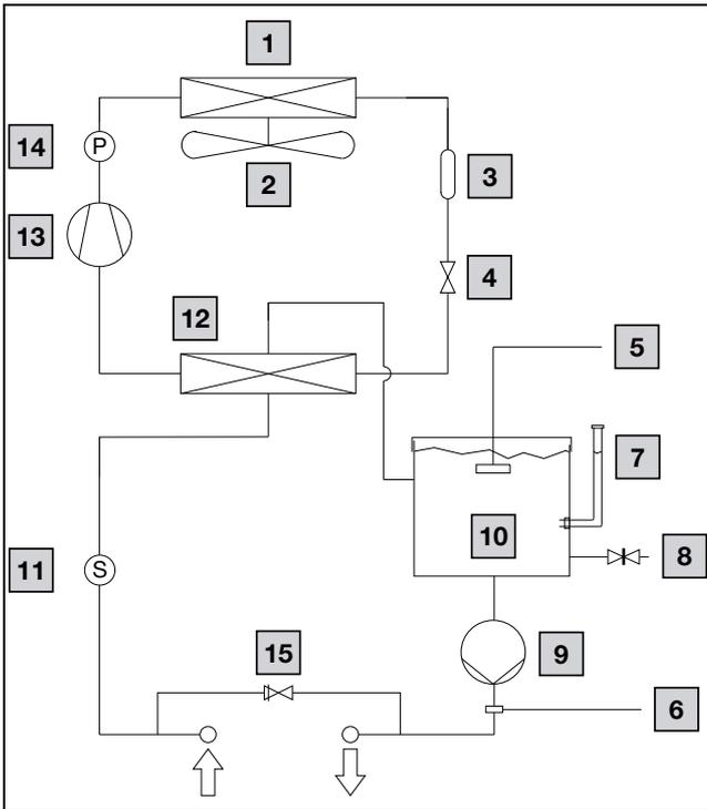
Fig. 9: Schematic diagram of refrigerant circuit
