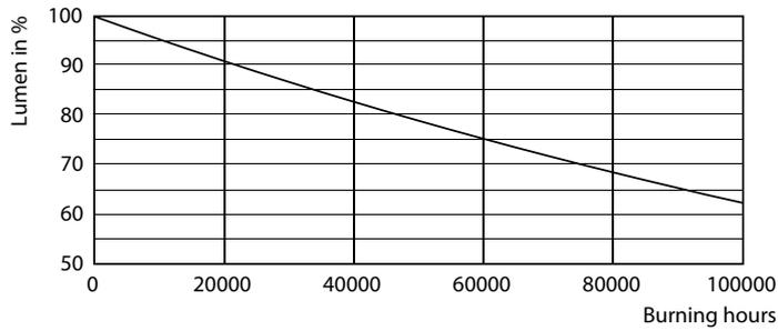
Lumen Maintenance Diagram - LEDtube Connected IA 1200mm 15.6W840
