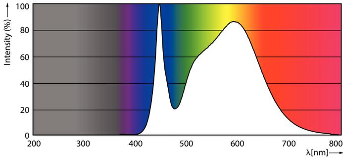
Spectral Power Distribution Colour - LEDtube Connected IA 1200mm
