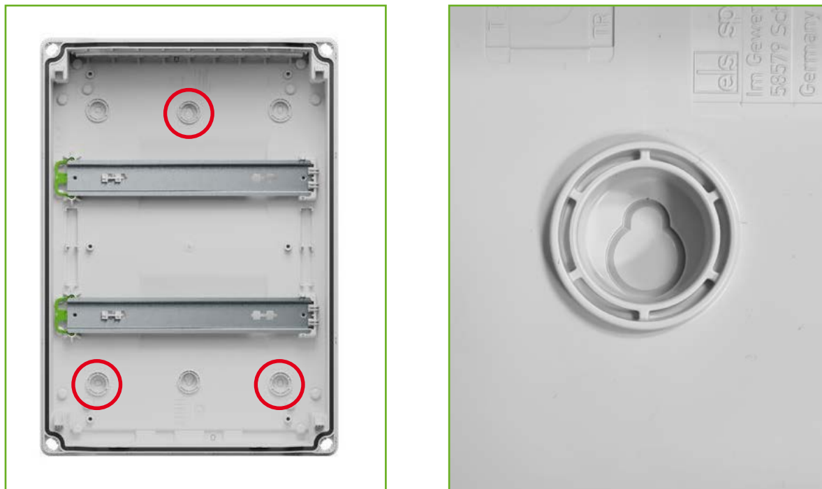
Figure 23: Fastening points 3-point installation, keyhole fastening
