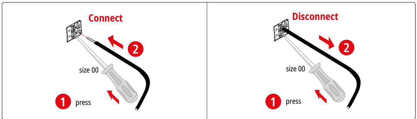
Figure 7 Connection / disconnection of the control lines
