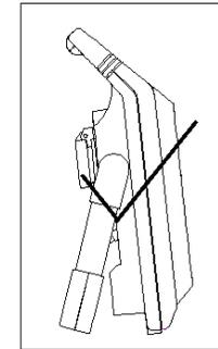
Secure the lamp against tipping - open the stand completely before using.
