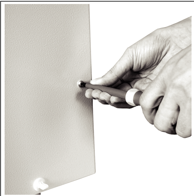
Fig. 27: Remove the assembly screws from the cover (loosen four screws)
