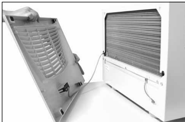
Fig. 20: Remove the louvred grille
