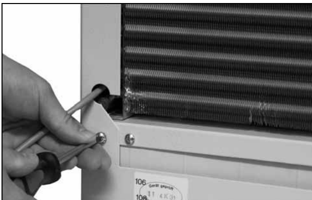
Fig. 23: Remove the assembly screws from the cover (loosen four screws)
