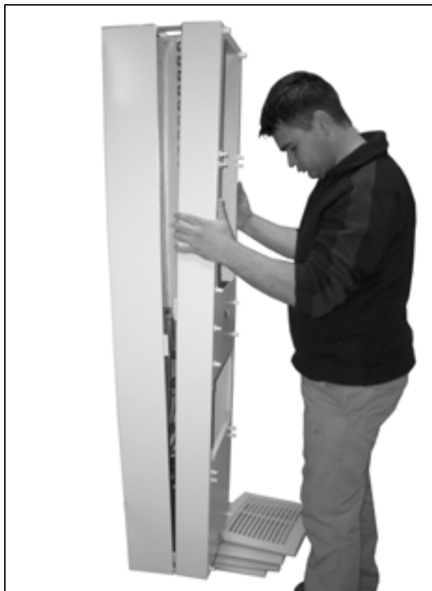
Fig. 76: Remover a tampa
