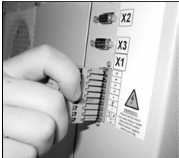
Fig. 28: Disconnect the mains plug
