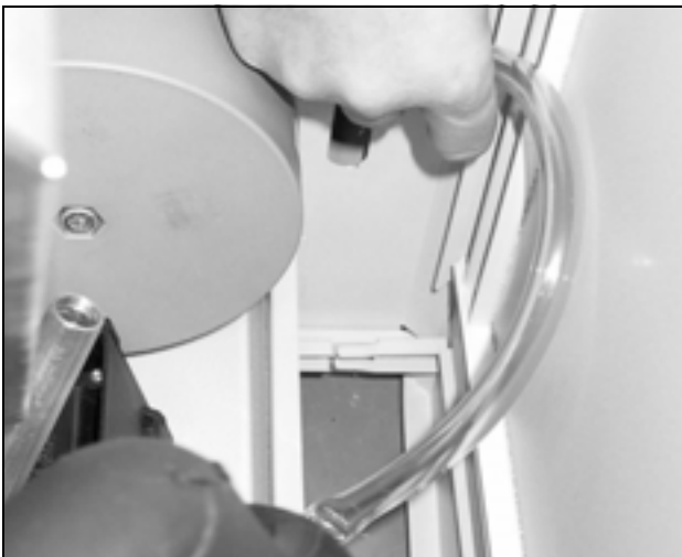
Fig. 9: Route the condensate discharge out of the unit
