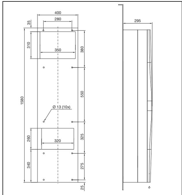
Fig. 96: 3328.xxx, 3329.xxx external mounting (except NEMA 4X devices)
