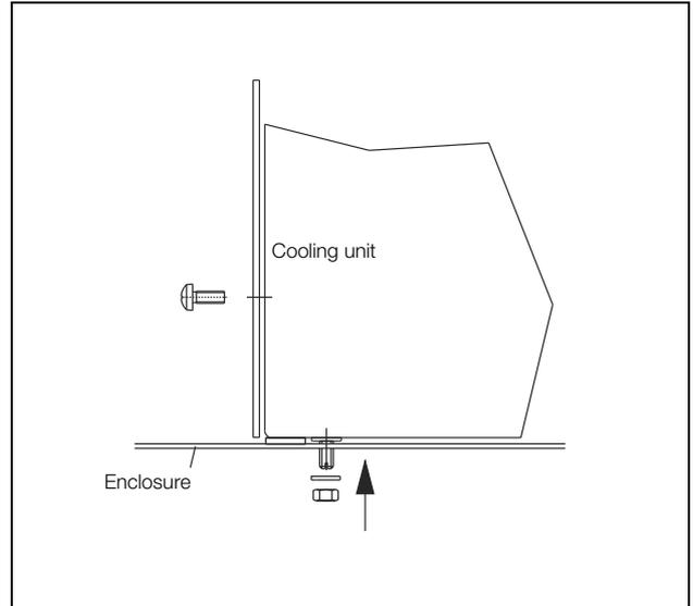
Fig. 78: Device mounting
