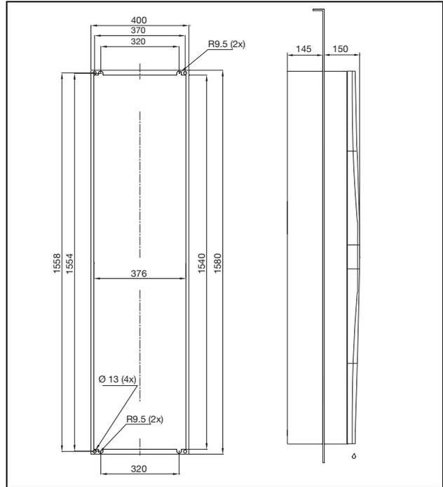
Fig. 103: 3328.xxx, 3329.xxx partial internal mounting
