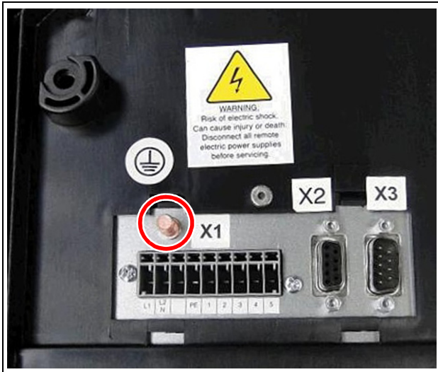
Fig. 11: Connection point, potential equalisation
