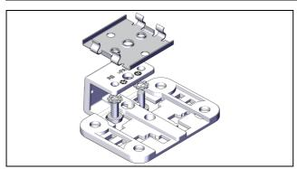
Fig. 5: Fastening the bracket to the spring clip
