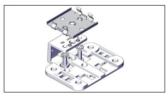
Fig. 5: Fastening the bracket to the spring clip
