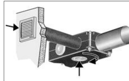
15. Replace the supply air or exhaust air inspection cover.
