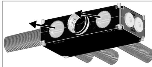
2. Remove the inspection cover at the air distributor (45° bayonet closure). Refer also to the housing "open/close" label.
