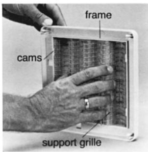
2. Take out support grille behind the cams and remove it from the filter frame together with the filter mat.
