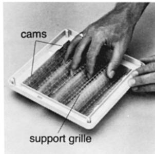
5. Push support grille below the cams at first on one side only. Then press it completely down onto the wave-shape and below the cams on the opposite side.
