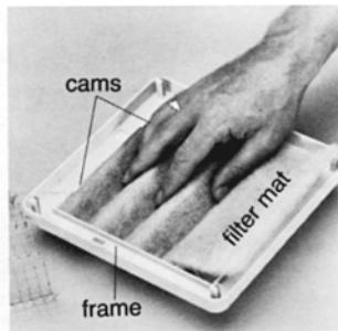
4. Press filter mat at first in the middle of the wave-shaped filter frame, then at the sides below the cams.
