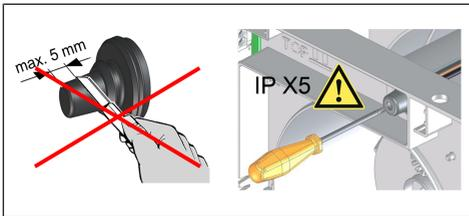
**⚠ DANGER** due to short circuit/fire if moisture penetrates into the terminal compartment. In the event of incorrect cable installation, the electronics cover cannot be used flat/sealed. Observe the permissible cable length in the terminal compartment. The grommet must be fitted firmly and tightly in the housing, even with the power cable.
