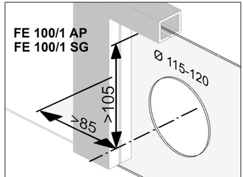
1. Have the window pane cut-out fitted by a specialist. For wall/wood panel mounting, drill a cut-out.
