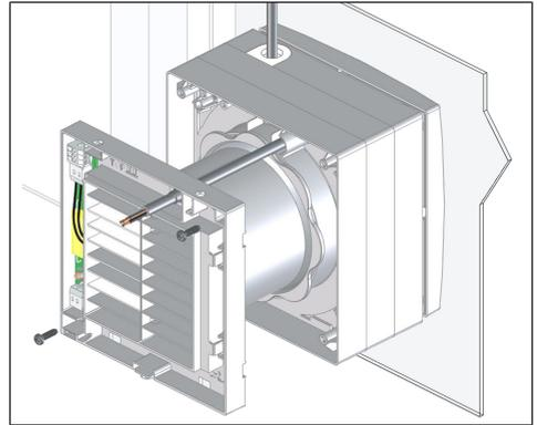
12. Screw the fan to the spacing frame with 2 screws.
