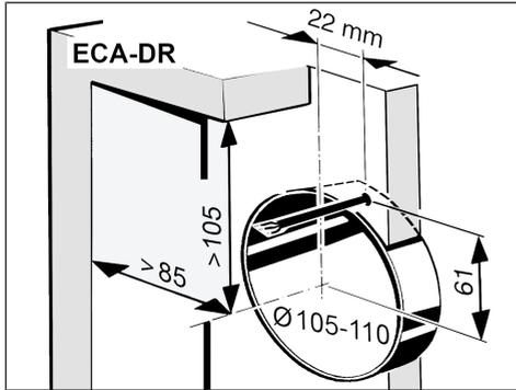
1. Drill wall breakthrough.
