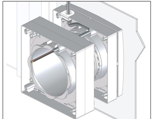
6. Push the power cable through the 10.5 mm hole in the other spacing frame.
