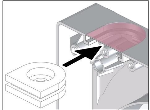
3. Cut out the opening provided in the housing on a spacing frame and insert the cable grommet.
