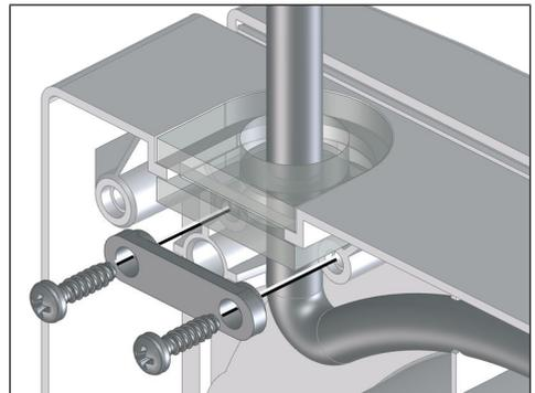
5. Fasten the power cable with the tension relief and route it to the right in the spacing frame.
