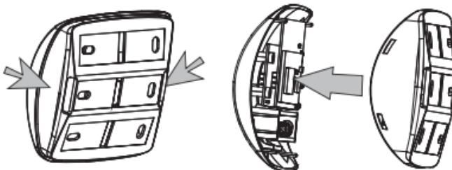
Fit the battery in the correct direction
