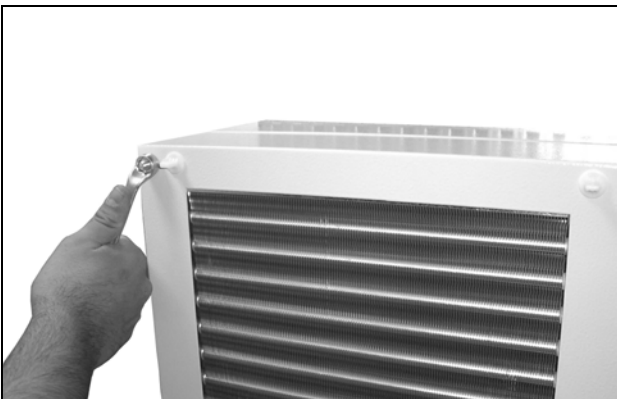
Fig. 44: Remover a tampa (soltar as quatro porcas)
