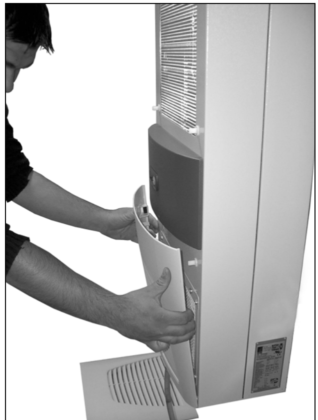
Fig. 36: Remover a grade inferior
