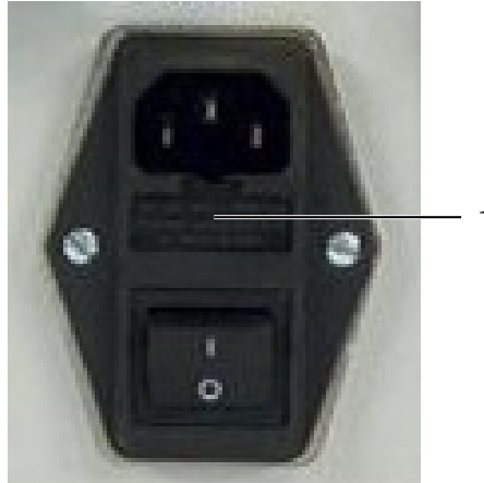
Fig. 27: Opening the fuse compartment
