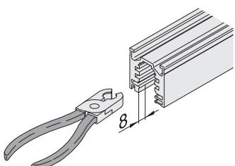
**EN** Cut to size of the track on site: N- and L-conductors must be cut back.
