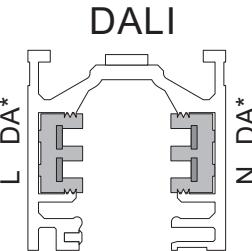
**EN** The adapter or track box of this luminaire/spotlight may **only be used in combination with the ZUMTOBEL L3 and DALI track and in DALI installations** corresponding with the diagram shown. Using these devices in tracks with standard 3-phase installations may damage the luminaire and is prohibited.
