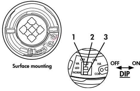
The DIP switch settings are overridden using the remote control.
