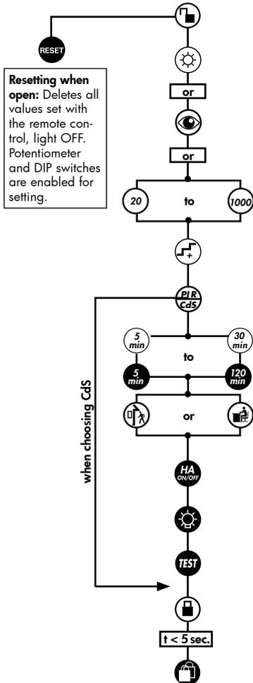
Unlocking device – Activation of the programming mode
