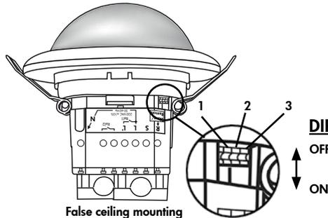
The DIP switch settings are overridden using the remote control.
