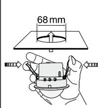
A circular opening of diameter 68 mm must first of all be produced in the ceiling.
