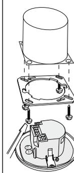
The detector can be installed in conventional inlet-sockets mounted on the ceiling. The assembly plate enclosed must be stripped off prior to installation and secured to the ceiling using 4 screws.
