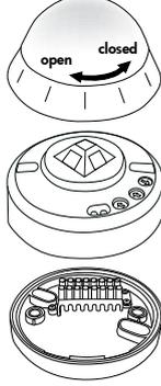
The detector must be installed on a solid and level surface. The circular cover ring must be removed prior to assembly. To do this, twist the lens anticlockwise through approximately 5° and lift off.
