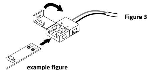
1. **Do not** remove the protection film at the connection position.
