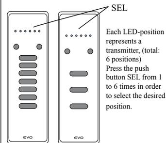
The selection remains memorised until the next variation, as well with turned-off transmitter; it is sufficient to press a channel push button to reactivate the last selection.
