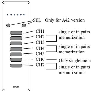
**TVEVO868A07/42 Separate push button Open-Stop-Close commands function**
