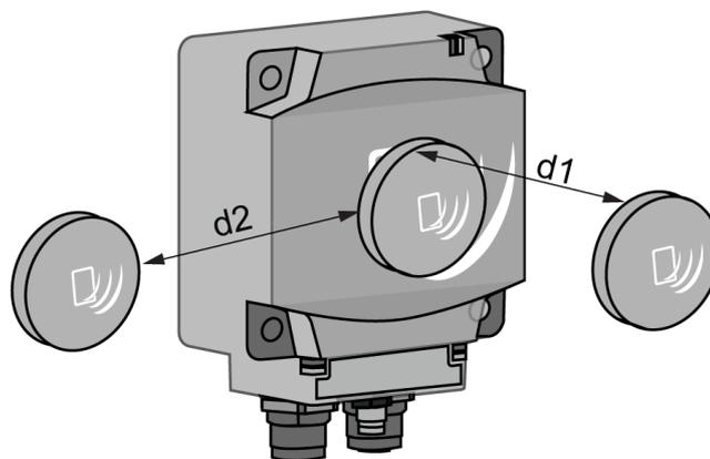
Minimum distances between 2 identical tags according to their positioning:
