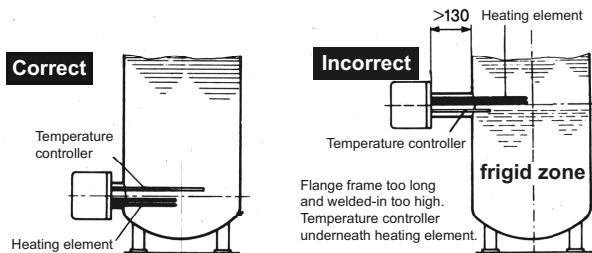
In order to ensure that temperature sensor and heating element reach far enough into the boiler, the flange frame must not be longer than 110 mm.
