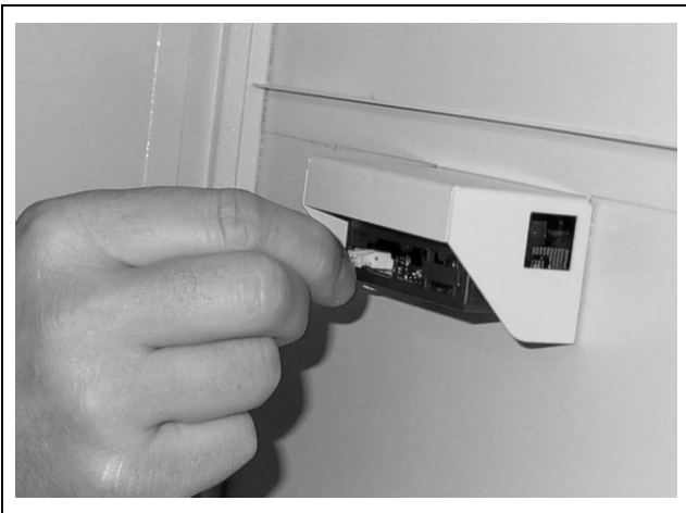
Fig. 13: Connect the display connection cable
