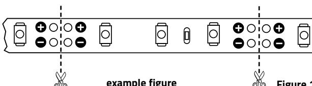
Separate the VARDIFLEX LED strip at the marked position. For a tightly assembled LED strip is a micro side cutter or an optional cutter required.
